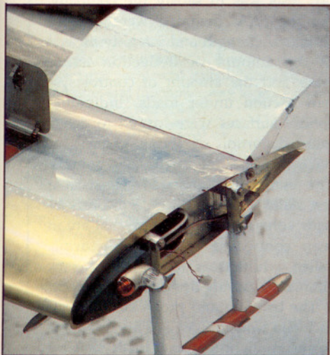
To achieve the goal of a cruise/stall speed ratio of 5:1, exquisite care was taken in flow control of the wings, which wear long Fowler flaps, equally long spoilers and tiny stub ailerons unloaded by anti-servo tabs.
